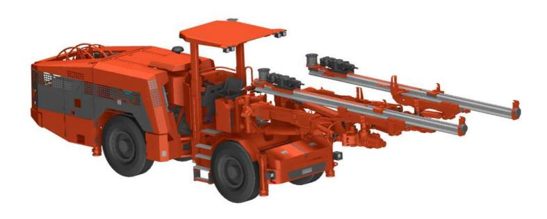
Sandvik DD421-60 is a two boom electro hydraulic jumbo for fast and accurate drilling in drifting and tunneling of 8-60 m<sup>2</sup> cross sections.
